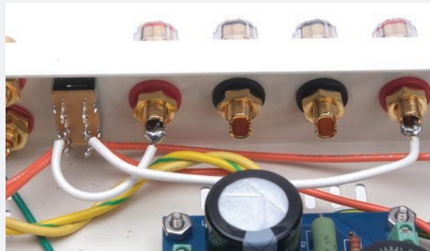
2. Use 2.5" and 5" pieces of 20 awg wire to connect the middle lugs to the red speaker binding posts.
