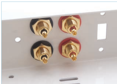
a. Mount the jacks so the solder cups face up, the insulating washers are centered, and secure with the first nut.
